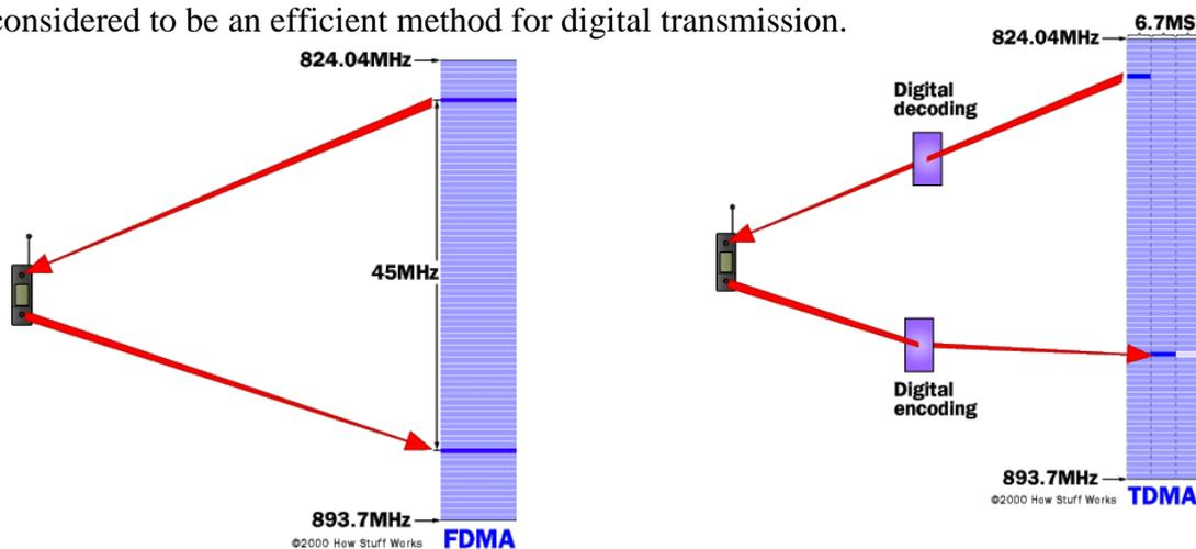
In FDMA, each phone uses a different frequency.
